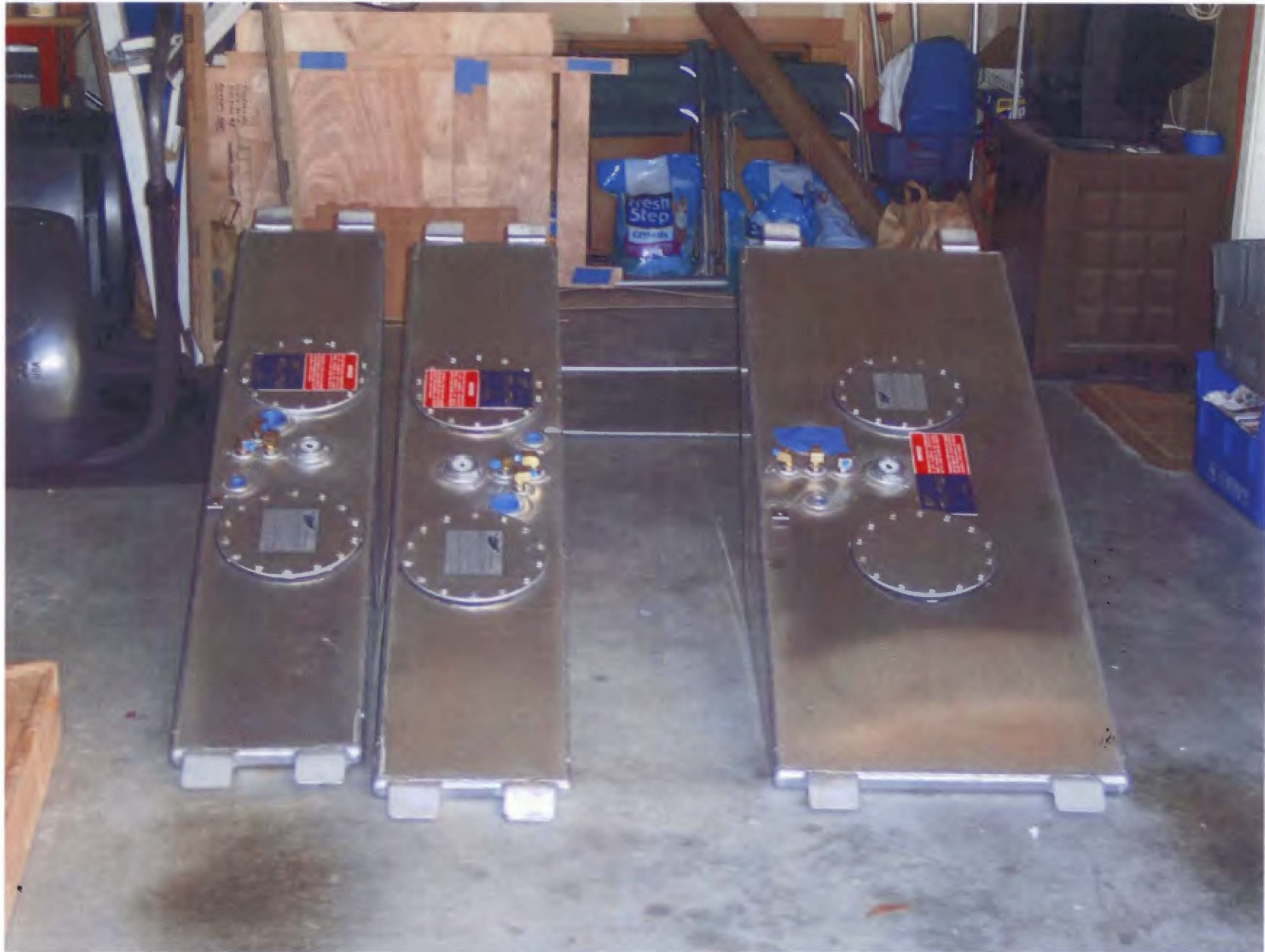
New aluminum tanks 22/22/44 gallon fabricated by S&P Sheet Metal
