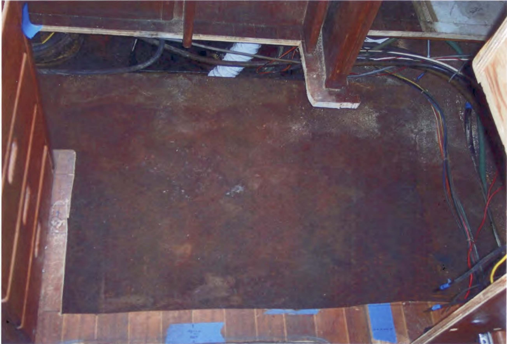
Quarter berth removed and cabin sole cut away over tank.
