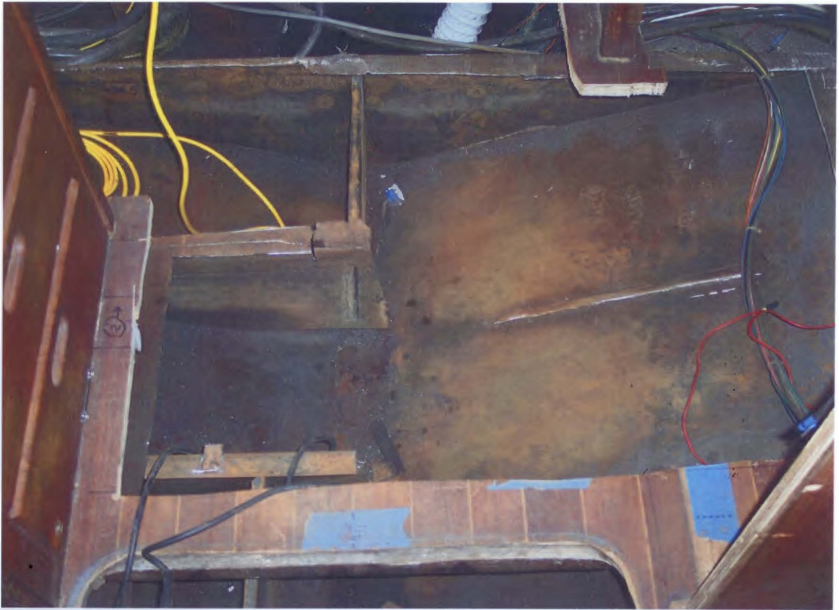
Cutting out the old tank.
