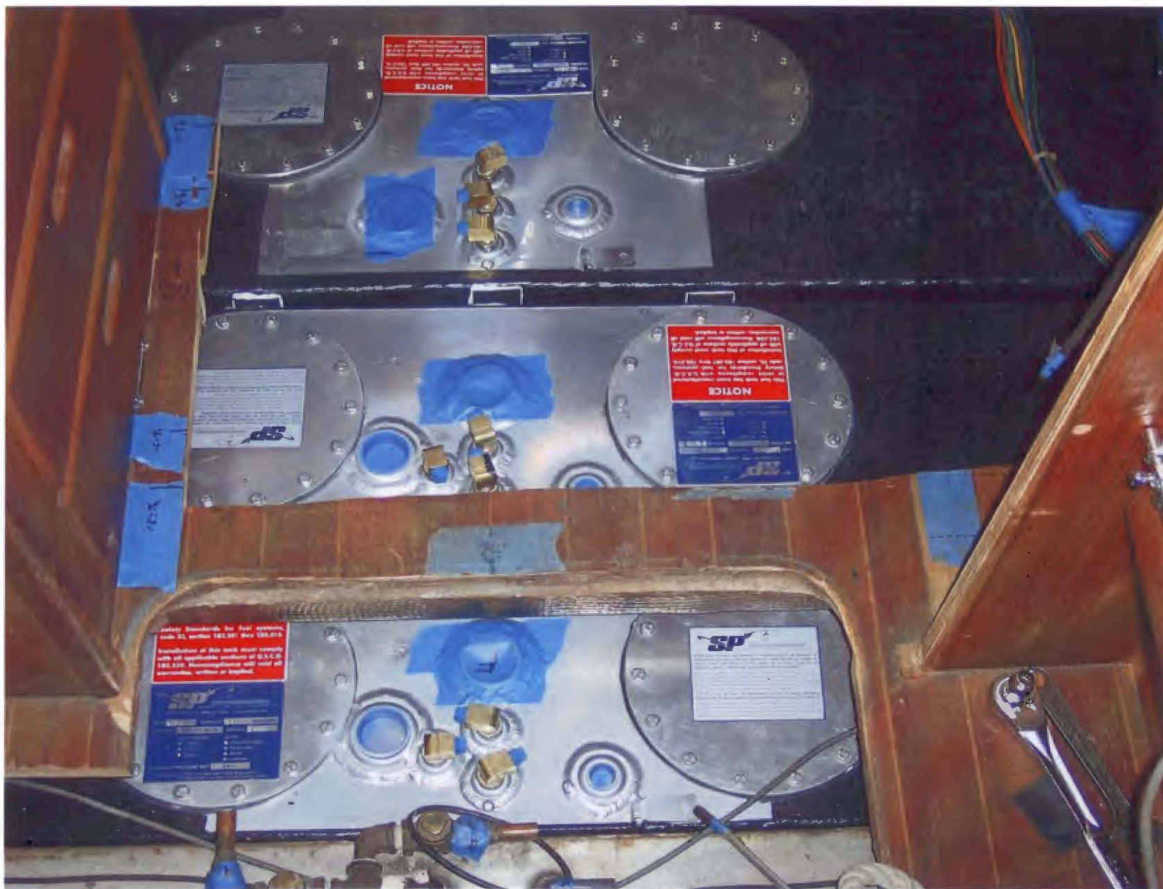
Tanks installed and ready for plumbing.
